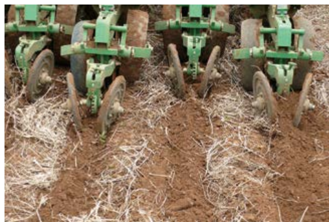
Figure 1.15: Direct seeding using rolling discs. In one operation, the seeds are directly placed into the opened soil which is compacted afterwards with the wheels of the same machine, Mato Grosso, Brazil. (Stefan Hohnwald)
