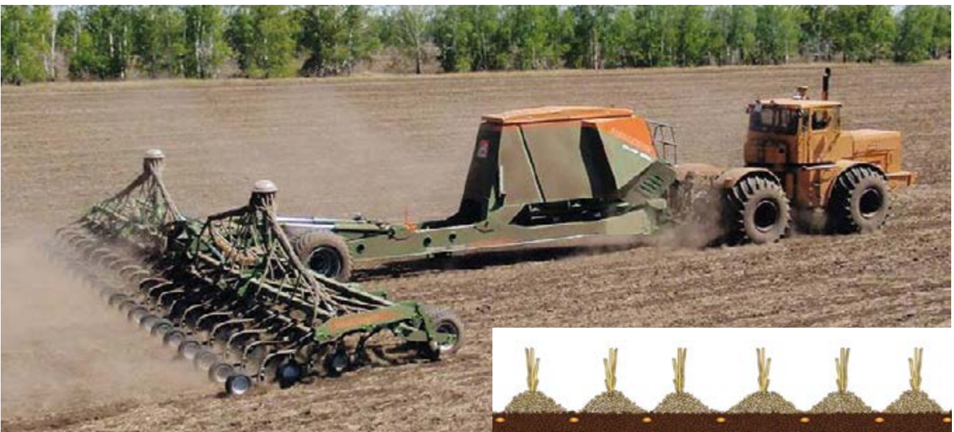
Figure 1.3: Russian tractor (Kirovets K700A) with an air seeder (direct seeder) 'Condor'. The scheme shows the seeds being placed between the lines of stubble in the wet soil. (photo: Tobias Meinel; illustration: Amazon-Werke)
