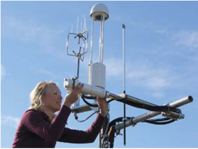
Flux station to measure CO 2 and CH 4 emissions in Siberia. (Elisa Fleischer)
