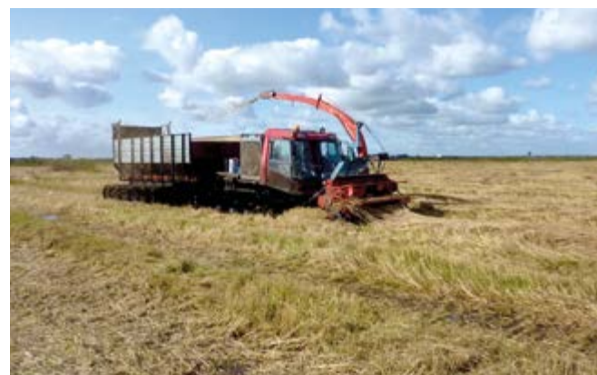
Figure 3.8: Prototype harvester for re-wetted areas. In order to retain some production from the wetlands part of the biomass is removed. (Wendelin Wichtmann)
