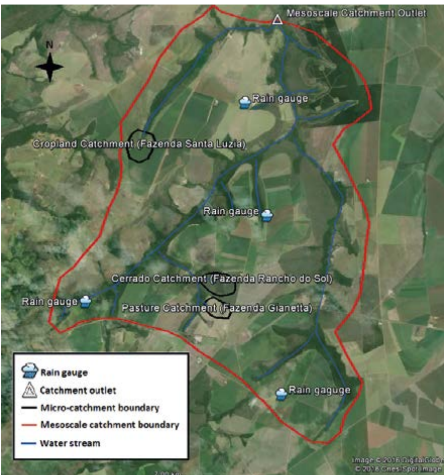
Figure 2.27: Tested micro-catchments (black circles) in a larger meso-catchment (red line) in Central Mato Grosso (Rio Das Mortes) with mixed land use: cropland catchment (Santa Luzia), Cerrado with mixed forest and shrub catchment (Fazenda Rancho de Sol), and pasture catchment (Fazenda Gianetta). (Carbiocial)
